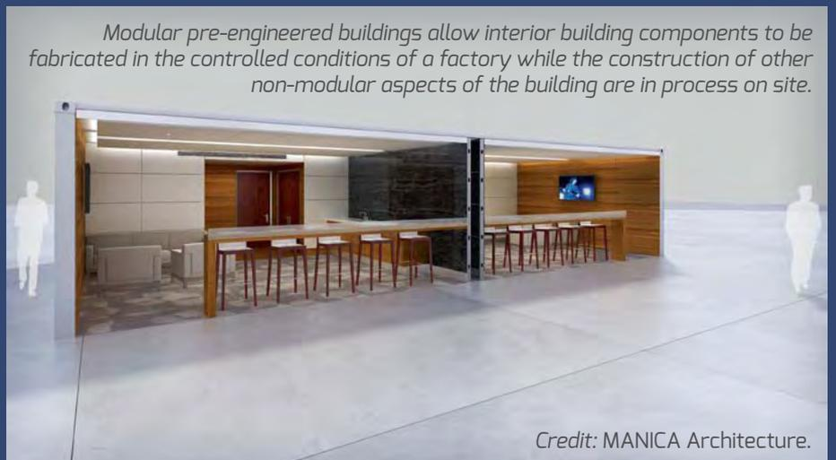
*Modular pre-engineered buildings allow interior building components to be fabricated in the controlled conditions of a factory while the construction of other non-modular aspects of the building are in process on site.*
